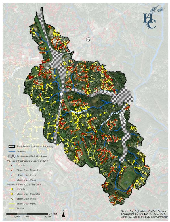
FIGURE 3.2. TIBER BRANCH WATERSHED STORM DRAIN MAPPING, PRE AND POST FIELD ASSESSMENT
