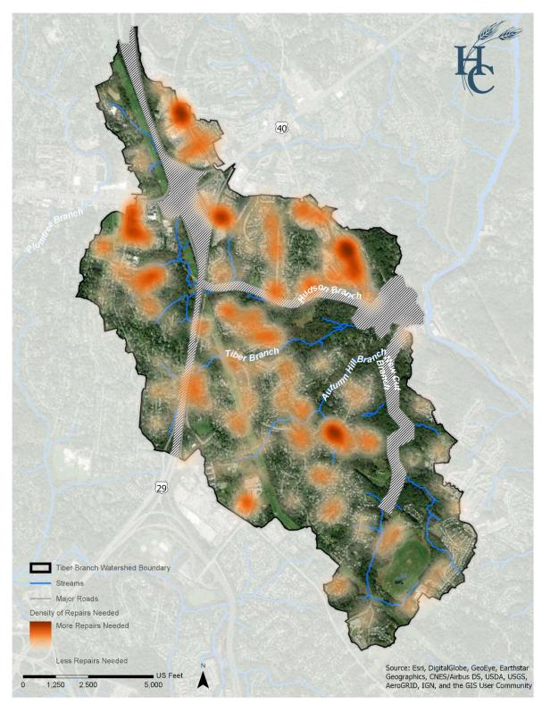
FIGURE 3.3. TIBER BRANCH WATERSHED STORM DRAIN CONDITION
