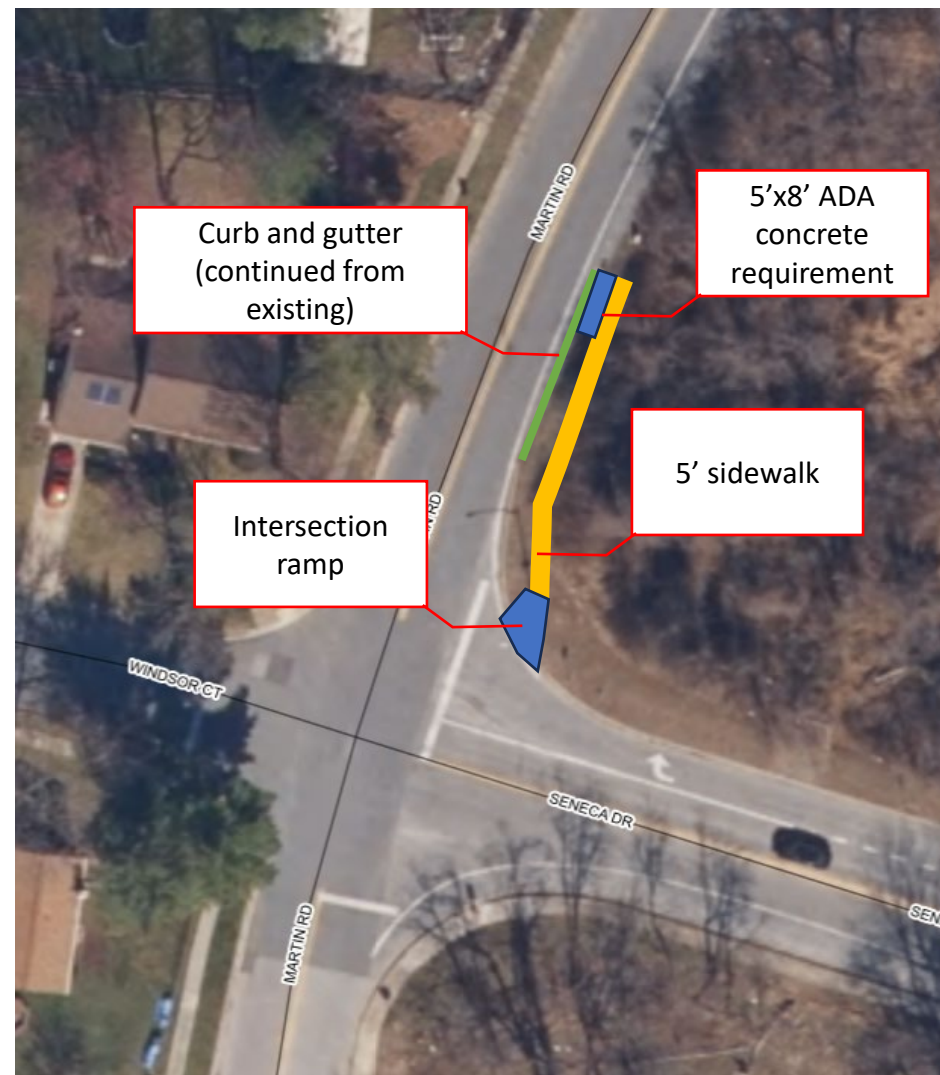
Required improvements for ADA compliance
