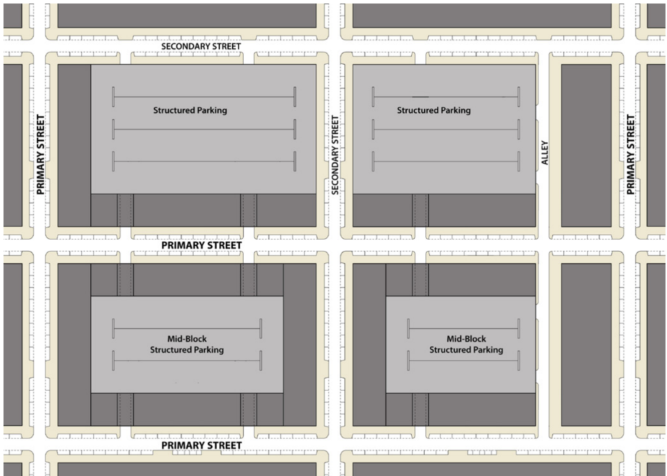
① Block Configuration Diagram - Various block configurations based on primary and secondary street frontage. For Primary and Secondary Streets, see Warfield Neighborhood Regulating Plan, p.11.
