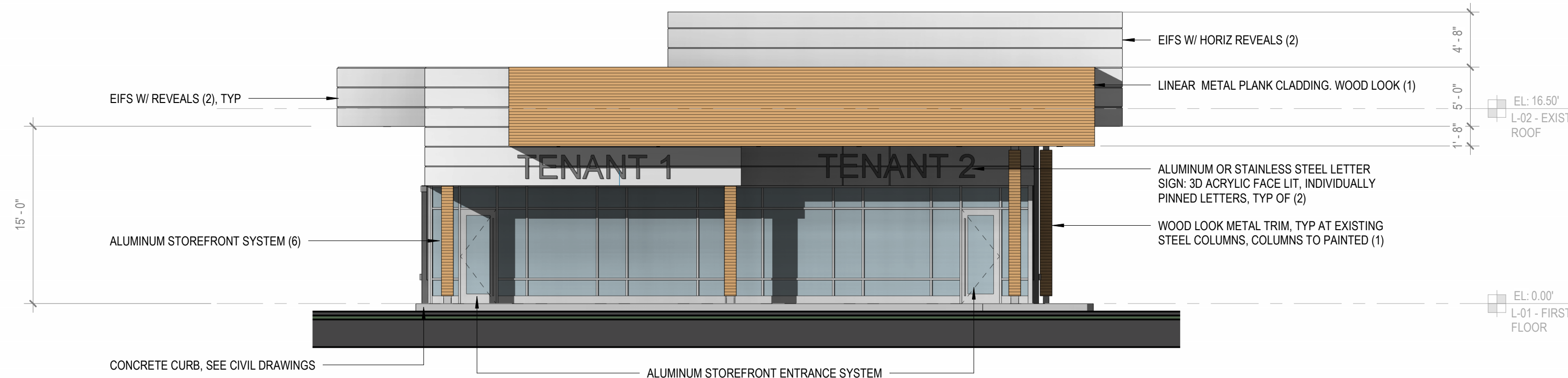
BUILDING ELEVATION SOUTH
