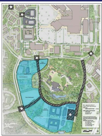
\*Alignment shown for the northsouth connector immediately south of Little Patuxent Parkway is an interim alignment. It is approved for development of the Crescent but is not the ultimate alignment shown at full buildout in the Downtown Columbia Plan.
