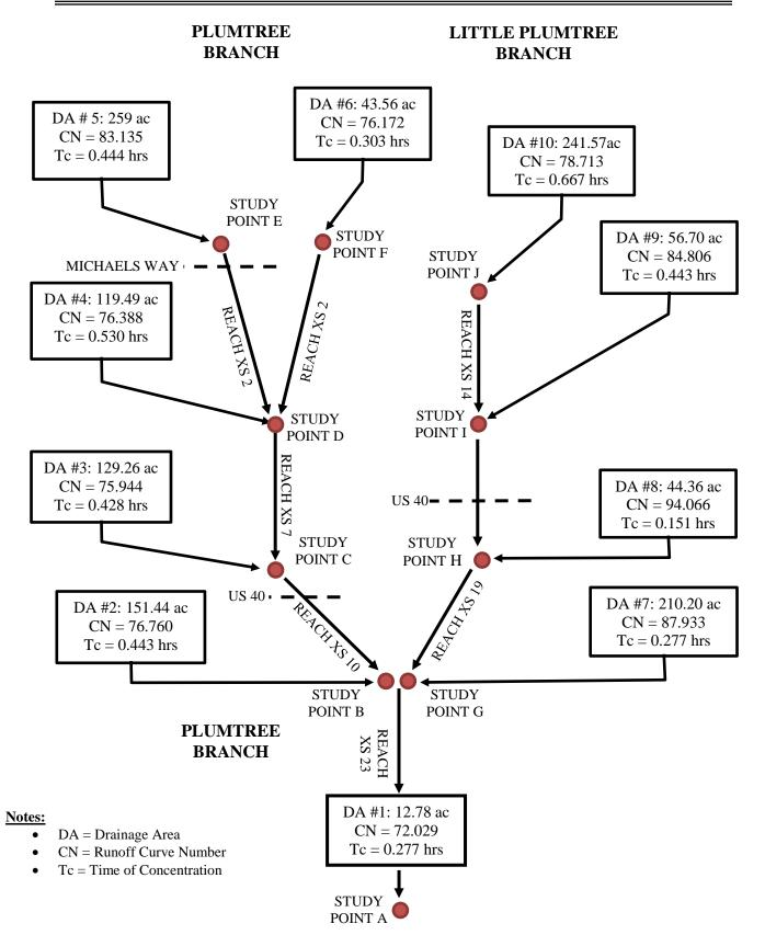
Figure 2.4: TR-20 Schematic for the Existing Conditions Hydrologic Analysis
