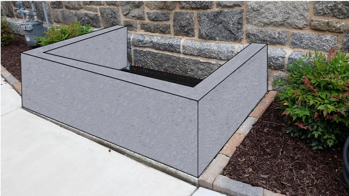
Rendering of Short CMU Wall Around NW Grate
