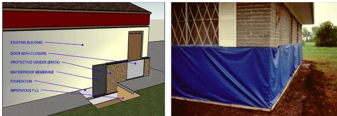
Figure 7-3: Temporary Dry Flood Proofing
