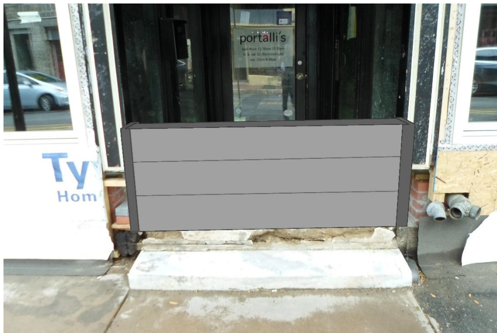
Rendering of Stoplog Door Closure
