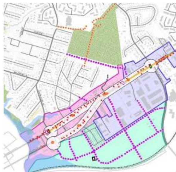
The area highlighted in white exhibits high proportions of crashes that may be related to driveways and high access densities. Access consolidation and orientation to local roads is recommended.
